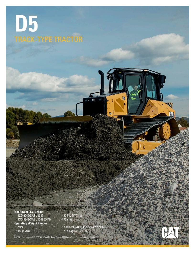
The new **Cat D5** succeeds the renowned D6N with superior performance and the broadest choice of technology features to help you get the most from your dozer. Nimble and responsive, it has power for dozing and finesse for grading. Fully automatic transmission gives you seamless acceleration, so you can get the job done quickly.
